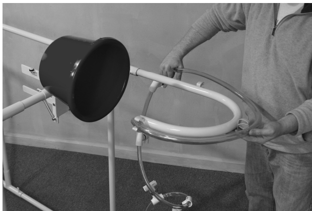
Attach filler tube. To the hook. Use the clips to route the filler tube along the frame.
