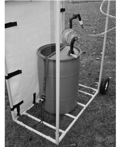
The drum can be attached to the base using the ratchet strap.
