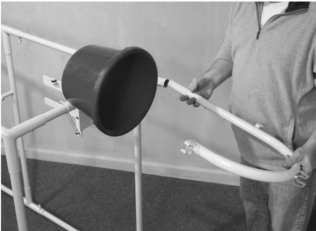
Insert filler tube hook and tighten.
