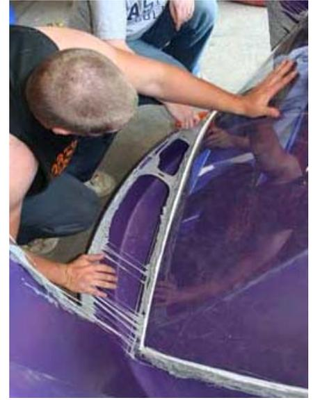
***This is a two person job (one person on the inside and one outside).*** The person on the outside pushes the window inward, while the inside person carefully cuts through the old grey butyl tape with a utility knife.
