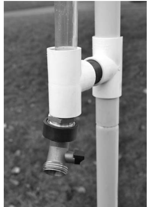
Attach the garden hose to the connector/valve.
