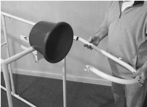
Insert filler tube hook and tighten.
