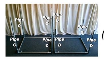
2. Insert (swedged) C Pipes into each corner of one square and the remaining (unswedged) D Pipes into the four courners of the other square.
