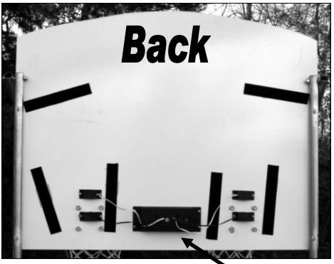
NOTE: Be sure to orient the digital display right side up, and attach the sensors with white wires to the top positions. The bottom wires (black) are positioned toward the outside of the scoreboard as shown.
